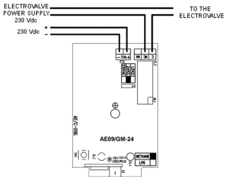
Electrovalves are usually open when being fed. When cutting-off the power supply blocks the gas flow and manual reset is required.
